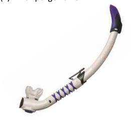
When using this type of snorkel you need less effort to remove the water from the mouthpiece because some quantity of water will be blown out from the purge non return valve which is placed next to the mouthpiece and therefore blow water out with less force than from the first type of snorkel, for the rest of the water to go out of the tube of the snorkel up to the top of part of it.
